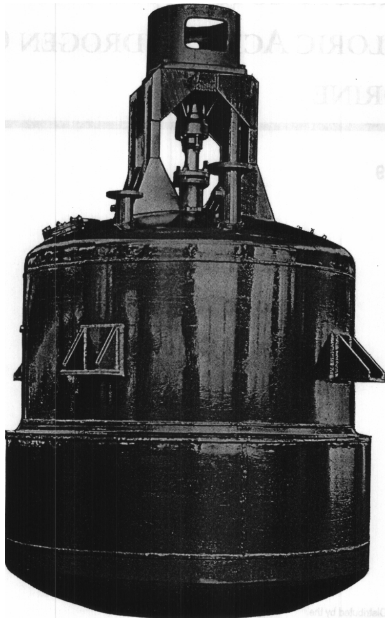
Nickel-clad steel jacketed reactor used for organic chlorinations. It was built in accordance with the A.P.I. A.S.M.E. code for unfired pressure vessels and operates at a temperature of 650° F, and pressures of 25 lb. per sq. in in the body and 125 lb per sq. in. in the jacket.
